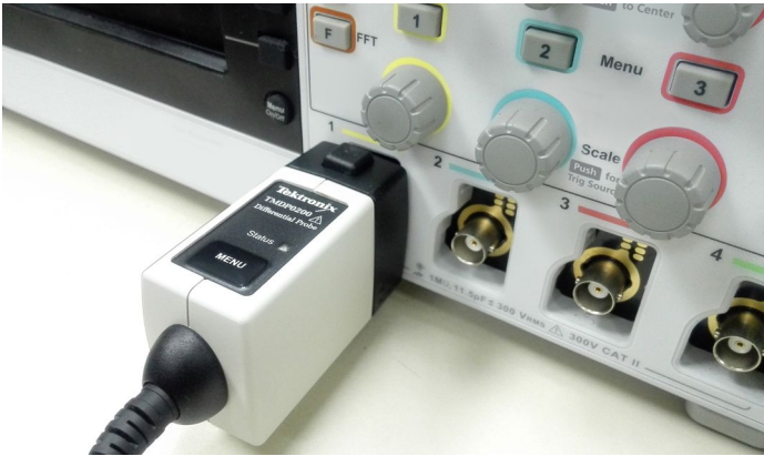
TekVPI probes communicate scale settings, ranges, and status to the TBS2000.
