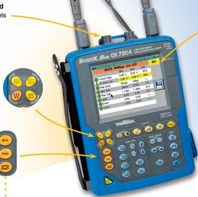
5.7" **TFT LCD colour touch screen** with LED backlighting, resolution 320 x 240 pixels
